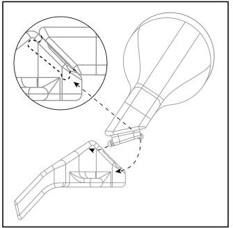
4. TO REMOVE, SQUEEZE NEAR THE CENTER OF THE UNDERSIDE WITH THUMB ON THE "R" OR "V" TO RELEASE BOTTOM TAB AND ROTATE OFF.
