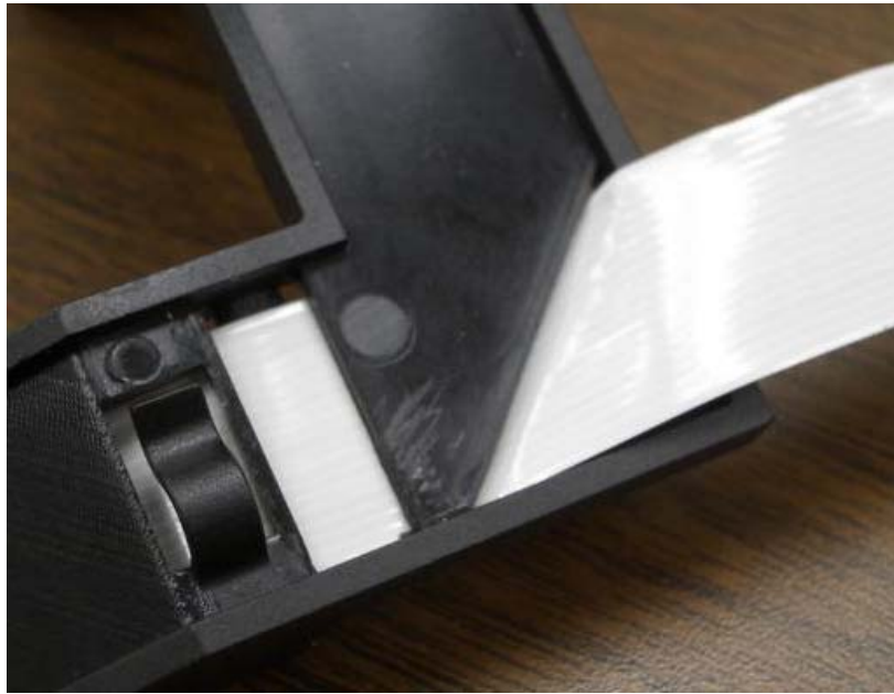
FIGURE 9: REMOVING SLACK FROM CABLE
