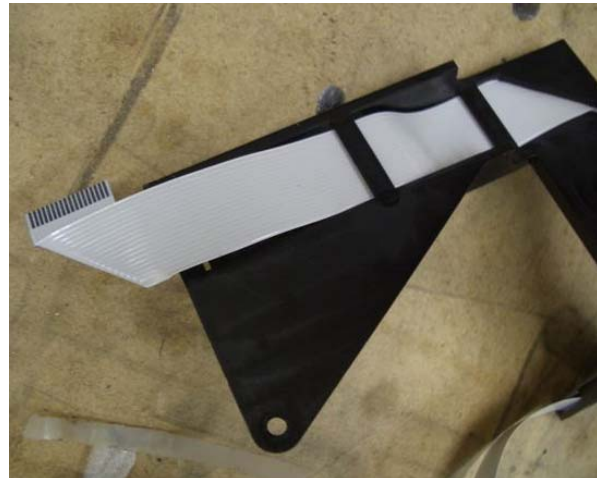
FIGURE 10: SETTING THE CABLE END POSITION
