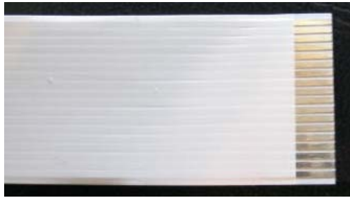
FIGURE 1: VIEW OF FFC CABLE END – STRIPPED SIDE
