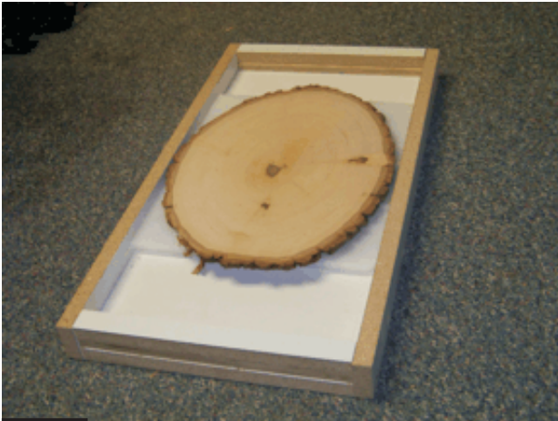
fig. 1 Jig Example for Carving Irregular Material
