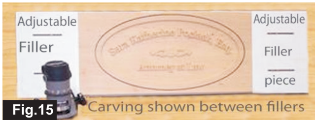
Figure 15 by Jim Krasselt (RouterJim) made a sled with adjustable end pieces to hold various sizes of carving material securely. Jim placed connection points periodically along the Carrier board so he can reposition the filler pieces to accommodate various lengths of carving material.
