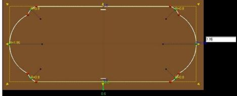
To change the radius on the vertical arcs, Left click and drag the left green node to the edge of the board.
