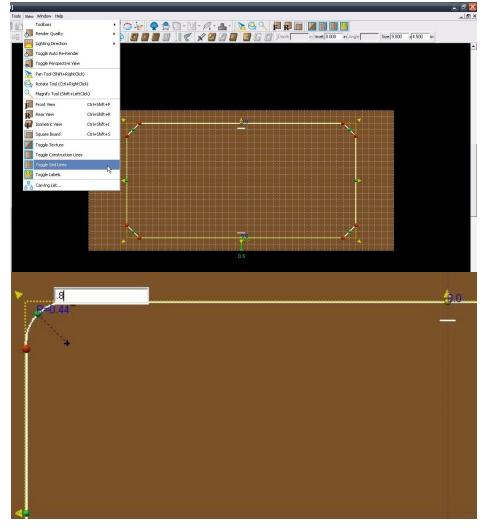
Repeat this step to constrain the three remaining corners to ".8".
