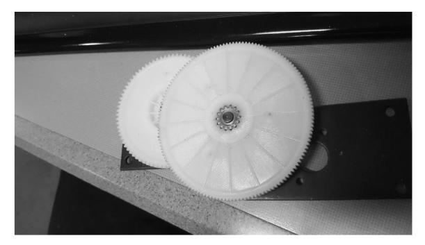
Once E-clip is removed, you can remove the Stage 1 gear from the plate. (Note: You may need to wiggle and turn this gear while pulling to remove it from the plate.)
