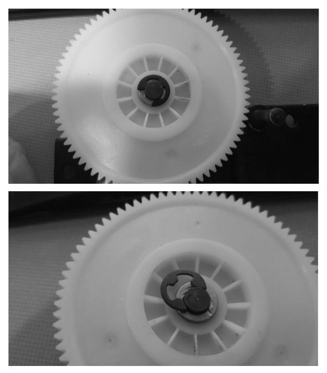
Note: You may need to wiggle and turn this gear while pulling to remove it from the plate.
