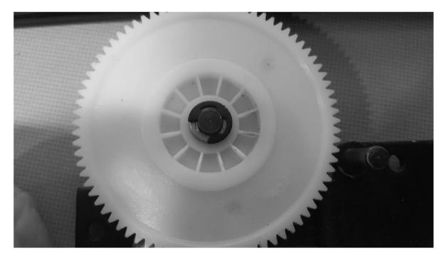
Put the new Stage 1 gear onto the shaft making sure the metal teeth on stage1 lines up with the stage 2 gear. Replace the E-clip as shown below using pliers.
