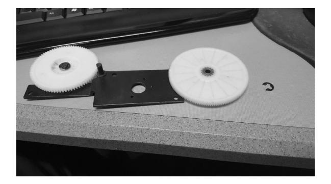
Repeat the same steps to remove the smaller Stage 2 gear. Do not lose e-clip.
