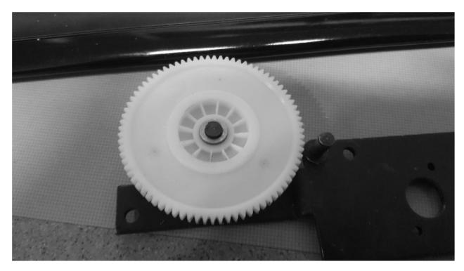
Below is the train plate without the Stage 1 or Stage 2 gears.
