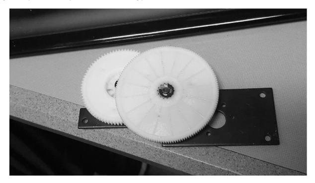
Apply grease to gear teeth, and rotate the gears by hand to distribute the grease around the teeth of each gear.
