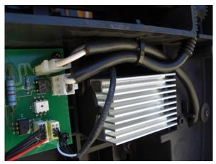
The final cable to disconnect is the four-wire DC power cable that connects the controller box to the power supply. Simply unplug the connector from the back end of the silver controller box.
