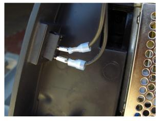
With the power cord free of the base we will disconnect the cable connecting the power supply and the X-Drive Electronics Board (green electronics board found directly behind the x-drive motor). Follow this cable starting at the power supply and clip the tie-wrap that secures it to the base wall. Disconnect the vertical two-pin connector found on the X-Drive Electronics Board.
