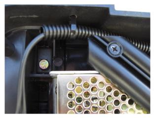
Finally, route the cable from the new power supply to the X-Drive Electronics board. Route the cable over the centerline of the machine (and across the tierod). Plug the cable into the vertical two pin connector on the board. It should snap into place.
