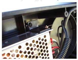
Next, place the diagonal brace with spacer into position on top of the power supply and start the screws (do not tighten).
