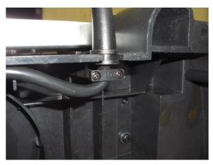
Connect the two spade connectors on the power cord to the ON/OFF switch. The connectors can be plugged to either switch terminal.
