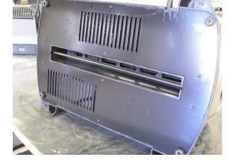
Next, disconnect the power cord from the machine (but leave it attached to the power supply). Remove the molded plastic bracket and two screws holding the power cord to the base of the machine.
