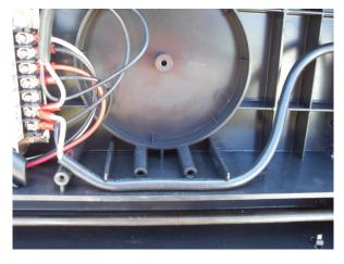
Replace the tie-wrap that secures the cable to the wall as it travels next to the x-drive motor.
