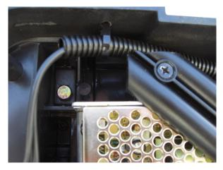
Unplug the two power cord wires from the back of the ON/OFF switch.
