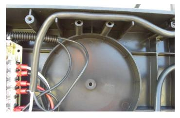
Replace the tie-wrap that secures the switch wires to the base.
