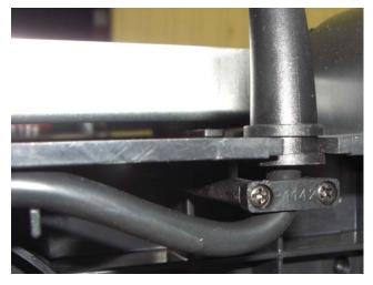
Follow the power cord wires from where they enter the base toward where they connect to the ON/OFF switch. Clip the tie-wrap that retains this cable to the wall of the base
