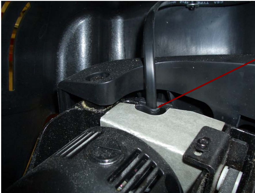
PICTURE 3: LOCATION OF AC INTERRUPT SWITCH CABLE WIRE RETAINER
