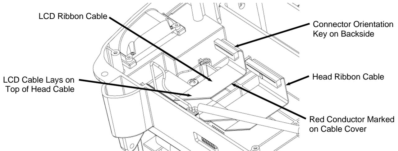
**FIGURE 17: POSITION AND ORIENTATION OF THE LCD RIBBON CABLE**
