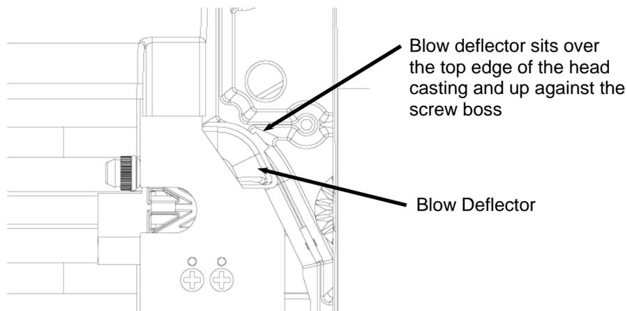
**FIGURE 21:** PLACEMENT OF THE BLOW DEFLECTOR - TOP
