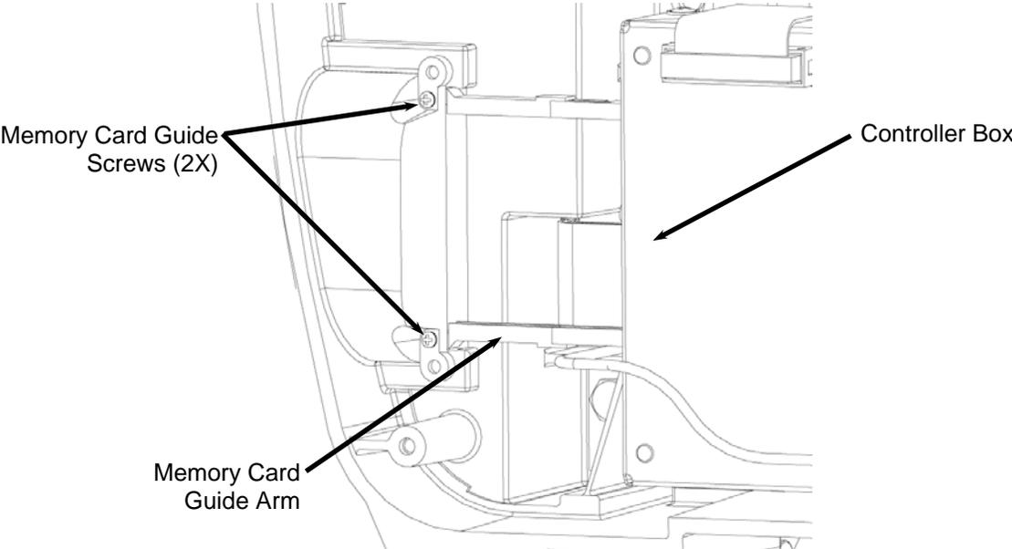
**FIGURE 15:** REMOVAL OF SCREWS SECURING THE MEMORY CARD GUIDE ARMS
