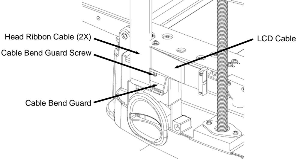
FIGURE 11: REMOVING THE BOTTOM RIBBON CABLE BEND GUARD
