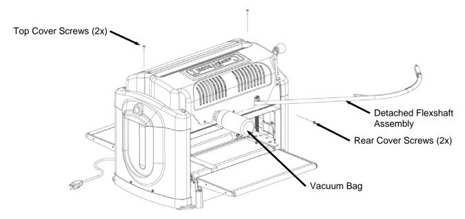
FIGURE 3: EXPLODED VIEW OF THE COVER SCREWS
