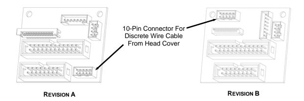
FIGURE 6: LOCATION OF CONNECTOR FOR HEAD COVER CABLE FOR THE EARLIER REVISION A AND LATER REVISION B MACHINES
