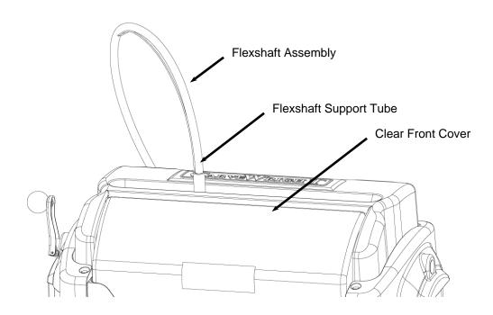
FIGURE 1: EXTERIOR VIEW OF THE FLEXSHAFT AND HEAD COVERS
