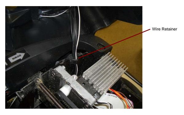
PICTURE 4: LOCATION OF HEAD CABLE HARNESS WIRE RETAINER
