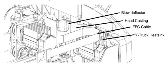
FIGURE 8: PLACEMENT OF THE BLOW DEFLECTOR - ISO
