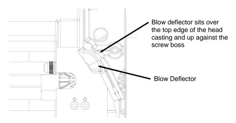
FIGURE 9: PLACEMENT OF THE BLOW DEFLECTOR - TOP
