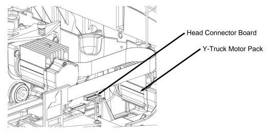
FIGURE 5: LOCATING THE HEAD CONNECTOR BOARD
