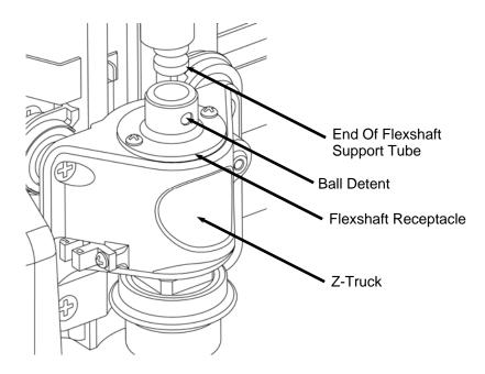
FIGURE 2: VIEW OF THE FLEXSHAFT CONNECTION TO THE Z-TRUCK
