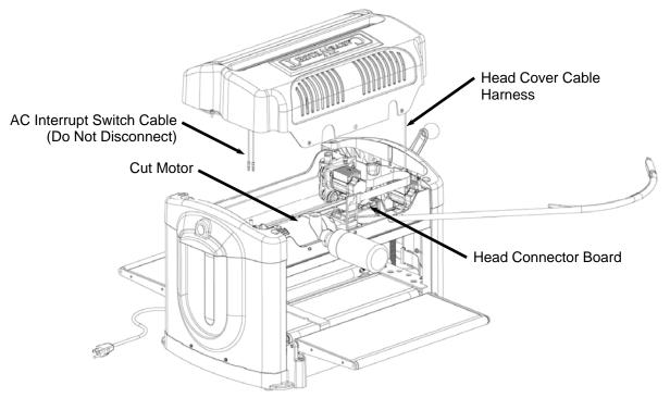
FIGURE 4: EXPLODED VIEW OF THE LIFTED COVER
