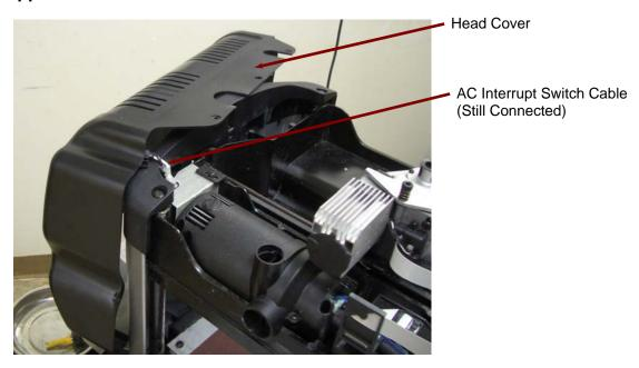
PICTURE 1: LAYING THE HEAD COVER OVER THE SIDE OF THE MACHINE
