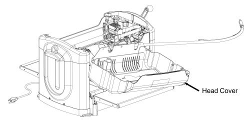
FIGURE 7: EXPLODED VIEW OF THE REMOVED COVER
