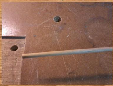
I flattend one side of the dowel a small amount to better fit the tab on the cover.
