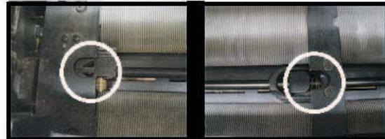
fig. 4a The jig's tabs fit into the two plate slots
