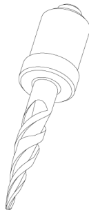
FIGURE 3: 1/16" CARVING BIT WITH PRESSED ON BUSHING
