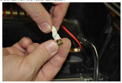
7. Place the Power Connector through the hole and replace the nut that you removed in step 6:
