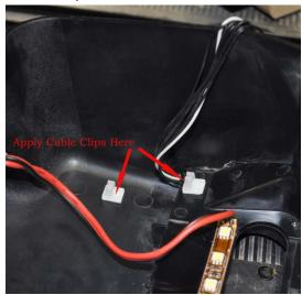
4. Clip the Power Cable into the Cable Clips
