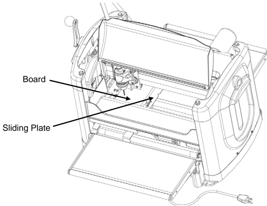
FIGURE 1: PROPERLY SET SLIDING PLATE
