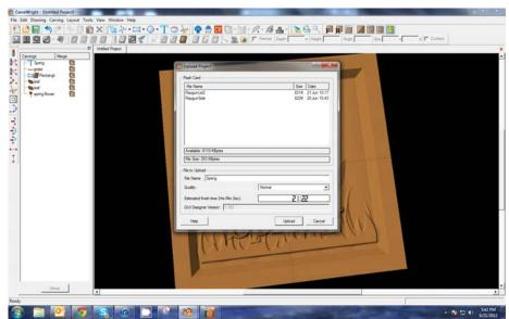
project. The more lines the better the surface finish. Make your decision based on material type, fondness of sanding vs. machine time, & test carve vs. final. Notice the estimated carving time differs by quality setting.
