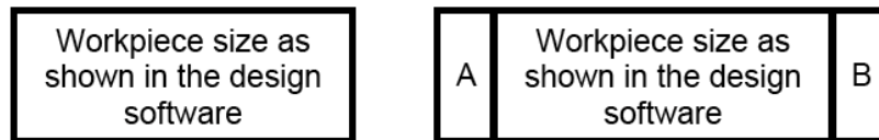
FIG 2.2.2 - 7 Inch Rule. A & B showing the extra 3 1/2 inches on both ends of the board
