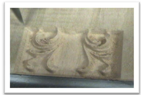
FIGURE I.6 RASTER CARVING LINE BY LINE
